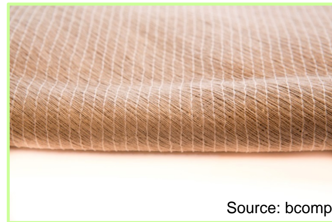
Woven and biax-reinforcement from flax fibers
